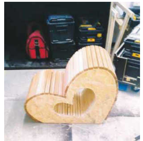
STEP 6. The ribs on the inside not only add to the aesthetic value but also give the chair additional support
